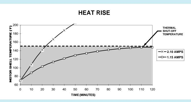
The shaded area in both the Performance Data and Heat Rise charts, contains pumps with current levels that are capable of running without periodic cool down. Pumps in this category will generally transfer more water over sustained periods than those in the unshaded areas, which are required to shut down while the motor cools. Some applications require maximum flows at high pressures for relatively short periods, however, so an explanation of thermal protection follows:
