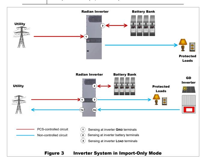
No-Exchange Mode: The inverter shall not exchange active power with the utility grid for either charging or discharging purposes. In the above figures, no current shall flow from point 1 to point 2. No current shall flow from point 2 to point 1. This operation may be engaged by setting the inverter to the *Mini Grid* AC input mode and setting *Charger AC Limit* to zero (among other options). In an AC-coupled installation, current may still be capable of flowing from point 3a to point 1a.
