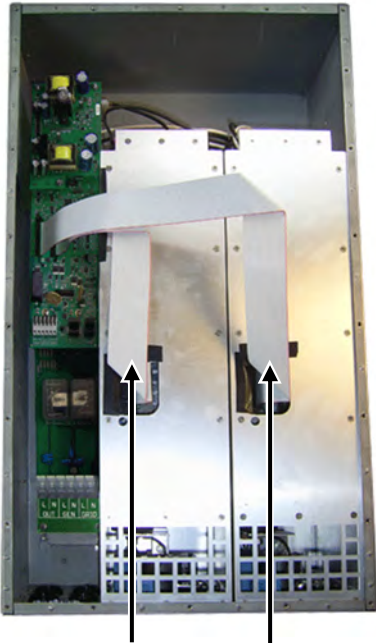
RIBBON CABLE: Connects the inverter's power modules and control board. See Warning below.
