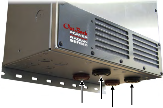
DC TERMINALS: Connects to the battery cables and DC system. There are two DC positive and two DC negative terminals. Each DC positive terminal requires separate cables and separate overcurrent protection. See page 26 for instructions.
